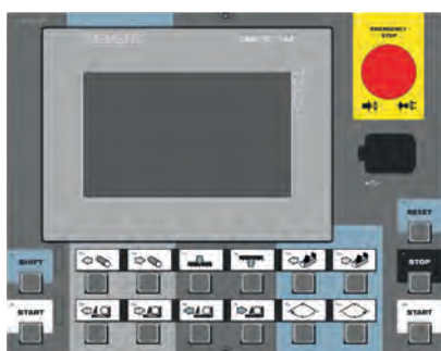
CONTROL PANEL: SIEMENS (X-CNC)
